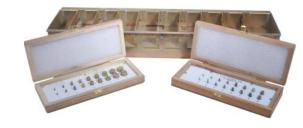
Average Least Dimension (ALD) device complete with ALD box - adjustable spacer – fine aggregates 2-9 mm, 1 x spacer set-fine aggregates spare case, spacer set extension 10-18 mm.
