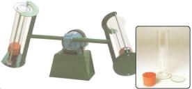
This method applies for soil containing upto 10% of particles retained on 37.5 mm sieve. The equipment is used to rotate two gas jars at approx. 50 R.P.M..Glass Jar is 1 litre in capacity with rubber bung.
