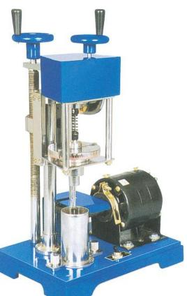
The vane shaft is attached through the hollow upper shaft to a resettable pointer, which indicates the angle indicates the angle of torque on a dial graduated in degree the dial reading multiplied by spring factor gives the torque a container for soil sample is also supplied & a sampling tube of 38mm. i.d. & 150mm long can also be used as container . Supplied with set of four springs, one each of approx. 2 kgs/cm2, 4kgs/cm2, 6 kgs/cm2 & 8kgs/cm2 complete as above in a wooden carrying case.
