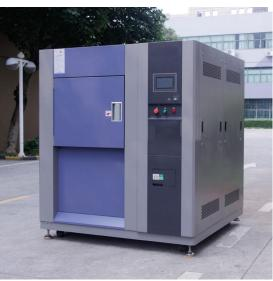
$\begin{tabular}{lll} KOMEG Model & KTS-150D \\ Temperature range hot zone & +60 ^{\circ}C to +200 ^{\circ}C \\ Temperature range cold zone & -80 ^{\circ}C to -10 ^{\circ}C \\ Temperature range test zone & -65 ^{\circ}C to +150 ^{\circ}C \\ \end{tabular}$
