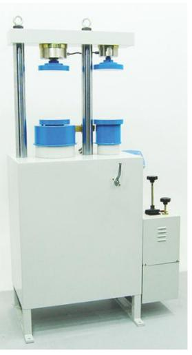
designed to supply the required oil to the load frames for loading. The power pack can load different frames with required pace rates. A rapid approach pump is supplied as standard. The power pack is equipped with a safety valve (maximum pressure valve) to avoid machine overloading.
