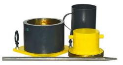
The Aggregate Crushing Value (ACV) test set provides a relative measure of the resistance of an aggregate to crushing under a gradually applied compressive load. Each set consists of steel cylinder, plunger, base plate, cylindrical measure and tamping rod. All parts of the apparatus are powder coated or galvanized steel, heat treated and ground before manufacturing to make it durable and reliable.
