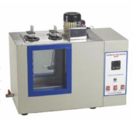
ASTM D 2171), which utilizes a vacuum slender viscometer. Complete absolute viscosity testing equipment adjusting to IS: 1206 (part II) method for testing tar and bitumen materials: determination of absolute viscosity with the accompanying segments:
