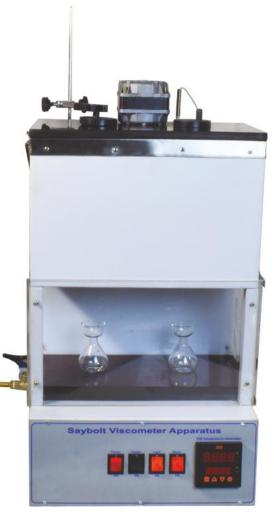
Pcs. ZI 4020D : Saybolt Viscosity Flask, Glass, 60 ml Dimensions : 450 x 300 x 550 mm Weight (approx.) : 10 Kg Power : 750 W
