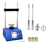
598. The hammer has a 4535 g sliding weight with a free fall of 457 mm 2 Nos.
