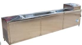
temperature is controlled by dual display microprocessor based auto tuning PID digital temp. Indicator cum controller. Control switches for motor, stirrer, heater and indicator lamps are fixed at a convenient place on the water bath. Complete with three briquette moulds and one base plate, all supply single phase. As per IS 1208.
