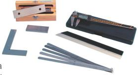
The appendix of EN 12390-1 Standard calls for a set of instruments to be used for dimensional and tolerance verification of the mould and the specimens got from the same.
