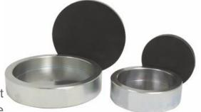
Pad-cap retainer rings hold neoprene pads that fit onto the ends of concrete test cylinders. Made from plated high-alloy steel to resist rust and deformation fatigue. Bearing surfaces machineplaned to within 0.002". Supplied two per set. Neoprene pad inserts are made from a tough elastomeric material that evens out and fills irregularities in the ends of concrete cylinders to assure even distribution of test loads for consistent results.
