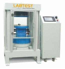
and the specimen is positioned and centered by the help of centering apparatus.
