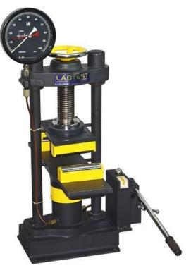
over travel switch protection to shut the machine down should maximum ram travel be reached. The return of the ram is done by dead weight to get maximum accuracy on the load measurement. All flexural frames have been designed to accept all the accessories for flexural and transverse tests
