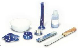
Shrinkage limit is the maximum water content at which a reduction in water content does not cause an appreciable reduction in volume of the Soil Mass. At shrinkage limit, on further reduction in water, air enters in to the voids of soils and thus keeps the volume constant.
