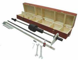
held vertically and the weight carefully raised to the handle limit and then allowed to fall onto the anvil. The equipment consist of the following replaceable parts
