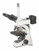
Metallurgical Microscope with Polarizing Attachments for study of Metallic surface under Polarized Light. Due to Polarizing effect the Metal surface shows the detailed surface properties with defects in colour patterns. This can not be achieved under normal light. If the surface of the metal is coated with Polarized light sensitive material the same can be studied for evenness of the distribution.
