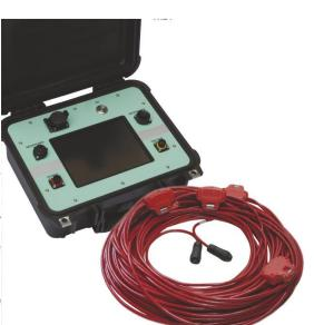
connection along the spreading: it will automatically recognise and count all geophones, performing the geophone tests and assuring you everything is OK before you start the acquisition. The real time noise monitor function will allow you to choose the best moment to shot.
